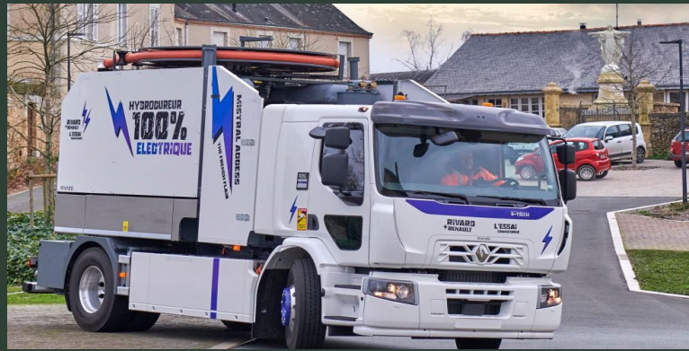
Rivard Mistral Access Electric Sewer Cleaning Truck
