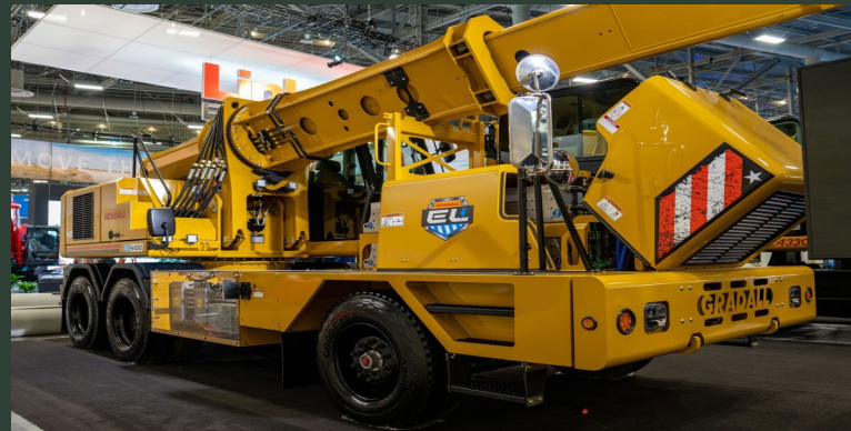
Gradall EL 4100 All Electric Excavator
