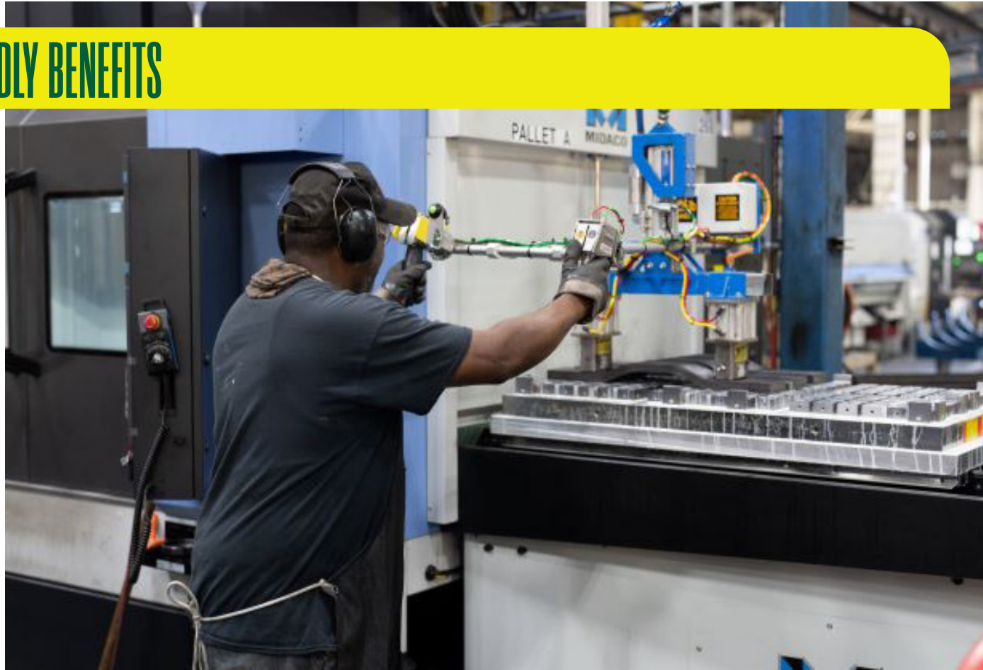
Robert Henderson operates a new CNC Blade Bar Mill machine at Bush Hog. The machine was purchased in 2022 to streamline milling efforts.
